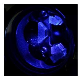
Figure 23.9: Picture of a strontium MOT operated at  $461\,\mathrm{nm}$ . The atomic cloud, which consists of about  $10^6$  atoms at  $5\,\mathrm{mK}$  temperature is visible as a diffuse spot located inside a three-mirror ring cavity.
