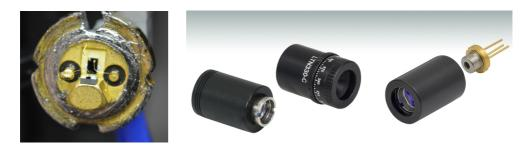
Figure 29.26: (Left) Laser diode with protective housing removed, e.g. using a can opener. (Right) Laser diode collimator.
