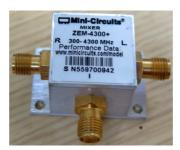
Figure 28.16: Picture of a radiofrequency mixer.
